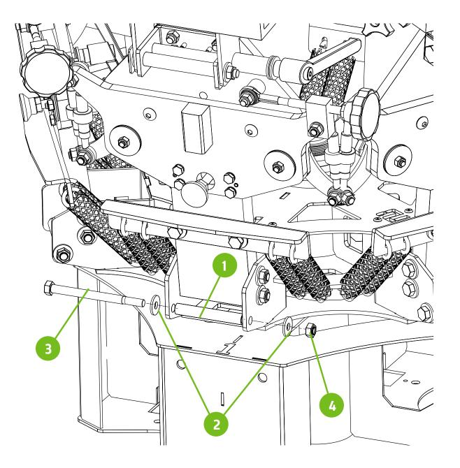
Install the Upper bumper bolt assemblies. No not overtighten hardware. Tighten just enough to hold in place.
