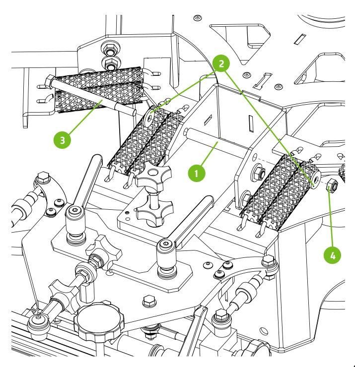
Install the print stations with supplied hardware. Ensure the number on the print station matches the number on the center rotary. Failure to due so, will shift the platens out of alignment.
