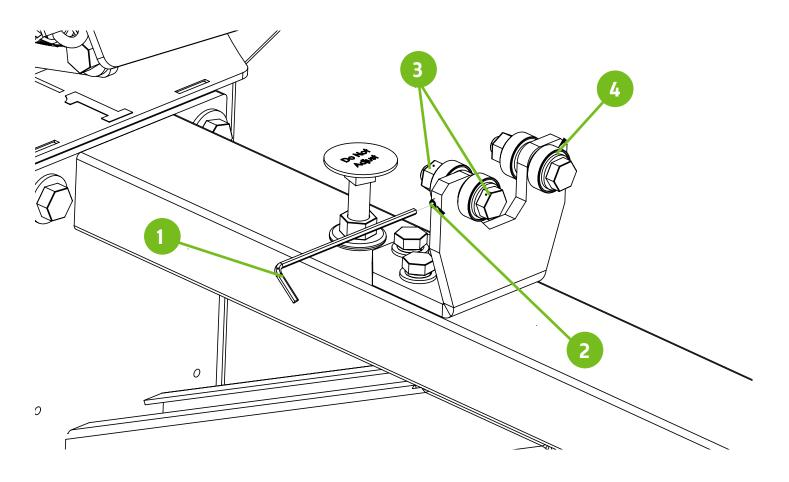
Level the screen clamping heads to the pallets. This one-time setting will work for the vast majority of printing jobs. Future adjustment may be required to accommodate "custom" platens that are much higher than standard.
