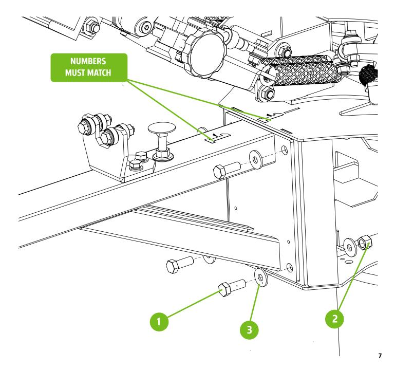
Install the 3/16" roll pins to locate the print station. Tap print station to align holes visually as close as you can. This is a factory setting that ensures your platens are aligned to each other. Tap them in approx. ½" with a hammer.
