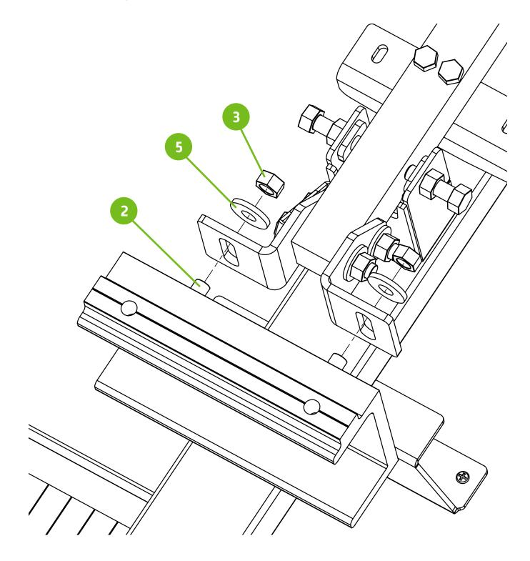
Install the screen clamp knobs into the screen clamp. Make sure the knob stud does not protrude beyond the lower clamping conical washer. Lock the nut together in opposing directions in order to fix the clamping nuts to the stud. Two 9/16 wrenches are required.
