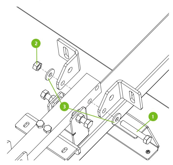
Install the upper off-contact bolt and retaining clip. This step may require you to rotate the lower bolt previously installed in order to fully seat the clip to the off contact bracket. One 9/16 wrench is required.
