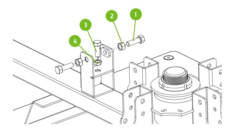
Set center Bolt 2-1/2" from top of bolt to top of base. Lock Jam nut to keep in place. Two 9/16" wrenches are required
