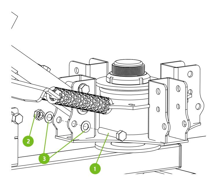
Adjust the side registration gate bolts and locking nuts. Center one of the print heads in the down position and align with the station arm. Snug the nylon bolts up to the color arm and lock the nuts against gate to hold in place. Two 9/16 wrenches are required.
