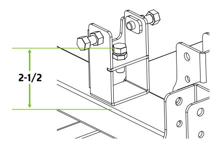
Install the Hinge hardware in the center of the three hinge pocket hole locations. Tighten the hardware to the point where there is some resistance but can still move up and down within the hinge pocket. Two 9/16" wrenches are required.
