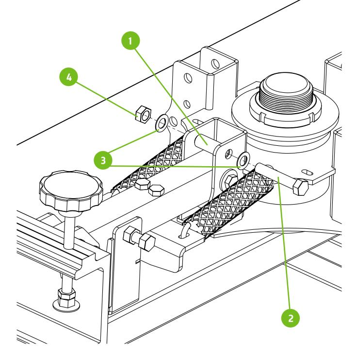
Install the lower safety stop bolt hardware. Make sure to install with the print head in the up position. **DO NOT** overtighten. Lightly snug nut to hinging pocket. Two 9/16 wrenches are required.
