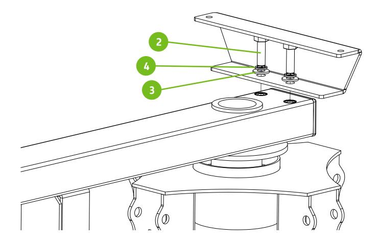
Mount the press base to the preferred tabletop surface. Shown with optional press cart/screen storage unit. Place front foot maximum 3" away from edge of tabletop surface for maximum platen adjustability. One Phillips head screwdriver is required.
