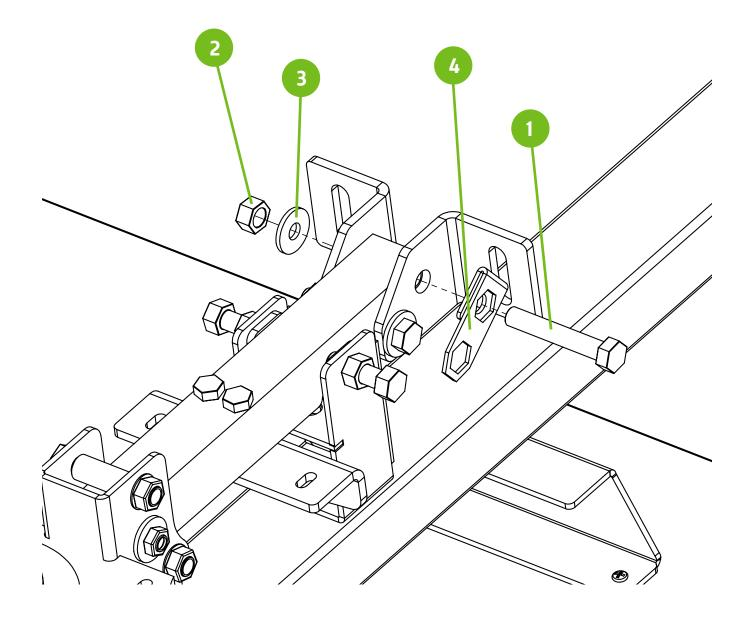
Install the off-contact bracket bolts into the screen clamp. Fully tighten the hardware at this step. One 9/16" wrench is required.
