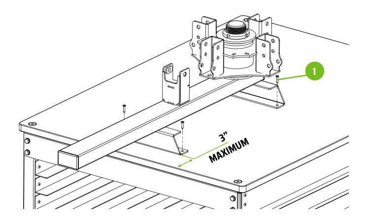
Install the gate hardware. Do not fully tighten the nylon side registration bolts at this step. Two 9/16" wrenches are required.
