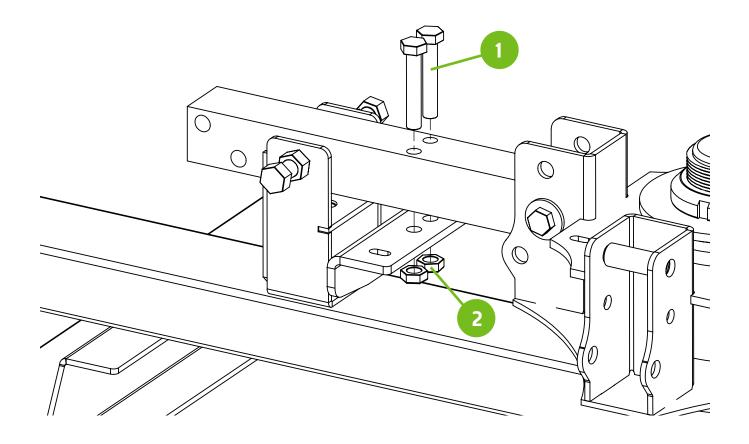
Install the lower pivot bolt into the off-contact brackets and the color arm lower hole. Do not fully tighten the hardware at this step.
