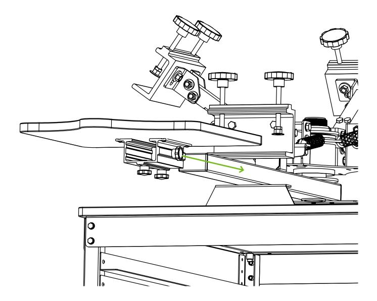
Set up screen. First lock the screen in place with the screen clamping knobs **(1)**. It is ideal to fully seat the screen into the back of the screen clamp as shown.
