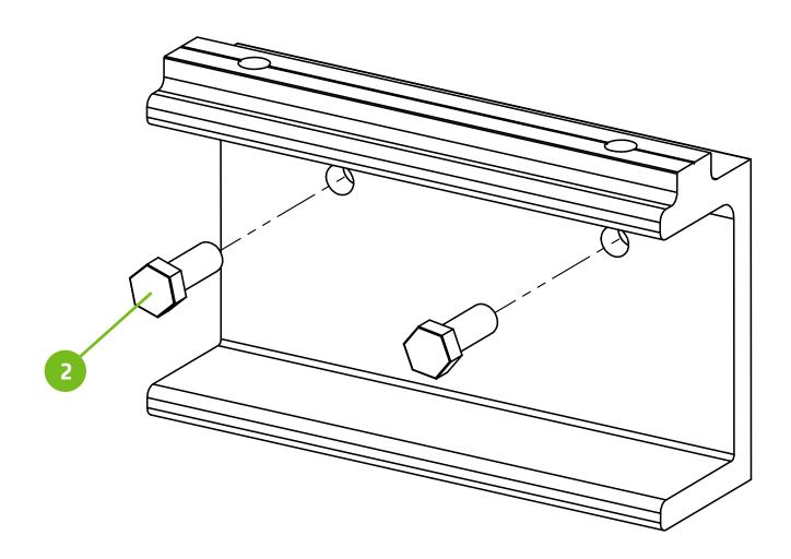
Attach the screen clamp onto the slotted off-contact brackets. This will be your up down adjustment for printing after final assembly. One 9/16" wrench is required.
