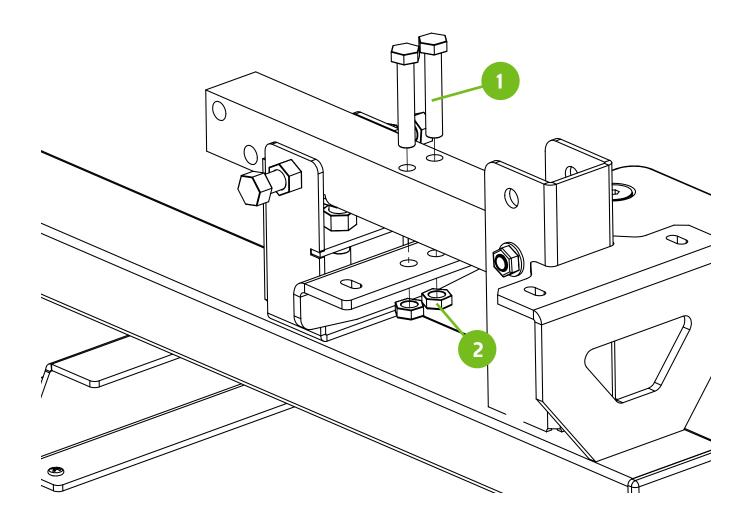
Install the lower pivot bolt into the off-contact brackets and the color arm lower hole. Do not fully tighten the hardware at this step.
