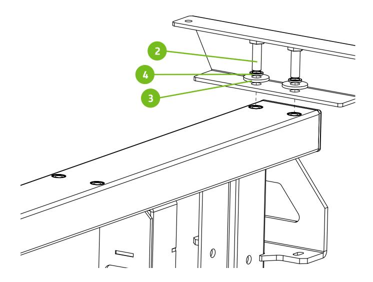
Mount the press base to the preferred tabletop surface. Shown with optional press cart/screen storage unit. Place front foot maximum 3" away from edge of tabletop surface for maximum platen adjustability. One Phillips head screwdriver is required.
