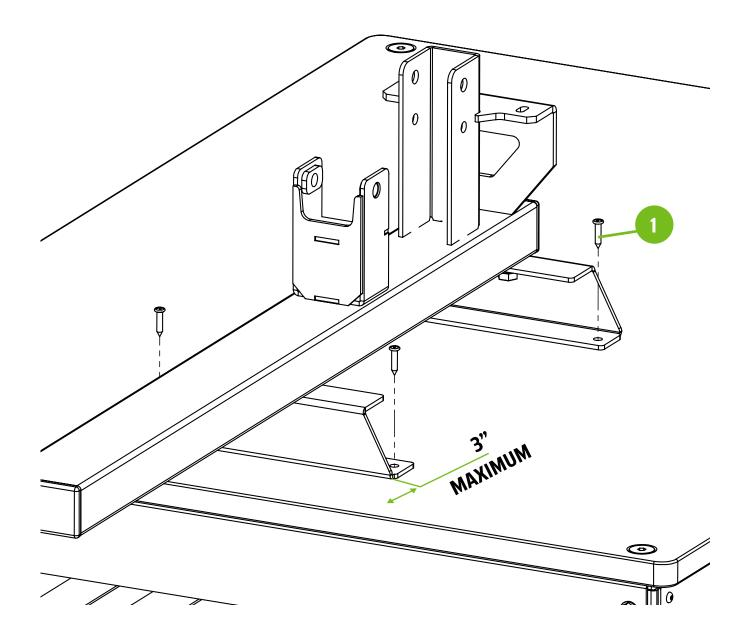
Install the gate hardware. Do not fully tighten the nylon side registration bolts at this step. Two 9/16" wrenches are required.
