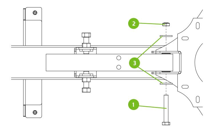
Attach the color arm spring plate to the color arm bar. Ensure that the spring plate is square with the color arm bar before final tightening. Two ½" wrenches are required.
