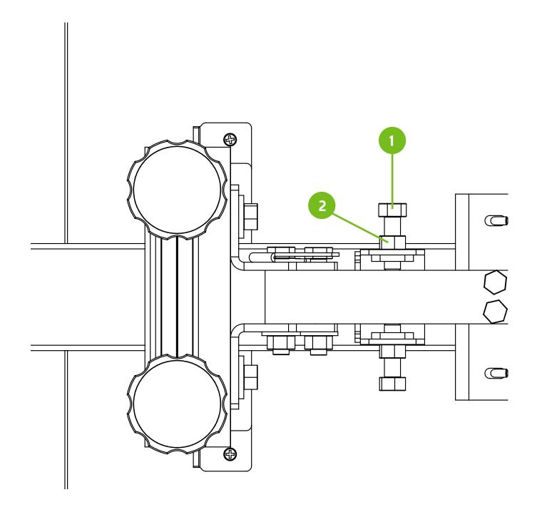
Install the Platen assembly to the station arm. Loosen the knobs before installation. It is adjustable front to back to help set the desired image placement on the garment. Lock in place with the three locking knobs tightly during print cycles.
