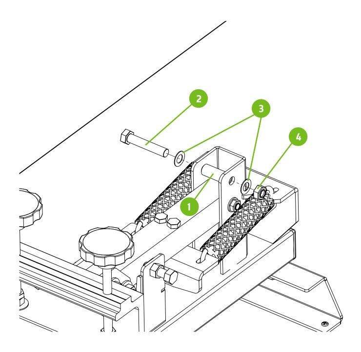
Adjust the side registration gate bolts and locking nuts. Center one of the print heads in the down position and align with the station arm. Snug the nylon bolts up to the color arm and lock the nuts against gate to hold in place. Two 9/16 wrenches are required.
