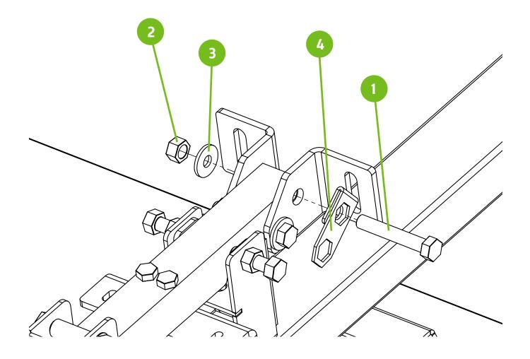
Install the off-contact bracket bolts into the screen clamp. Fully tighten the hardware at this step. One 9/16" wrench is required.
