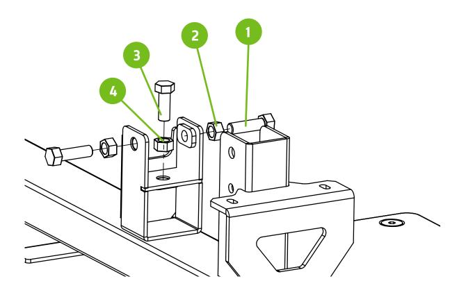
Set center Bolt 2-5/8" from top of bolt to top of base. Lock Jam nut to keep in place. Two 9/16" wrenches are required
