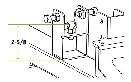
Install the Hinge hardware in the center of the three hinge pocket hole locations. Tighten the hardware to the point where there is some resistance but can still move up and down within the hinge pocket. Two 9/16" wrenches are required.
