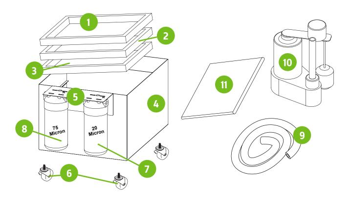
Fasten the casters to the base of your unit. Adding spacers between caster and caster mounts on body.
