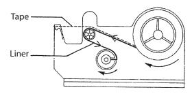
If the spool (1) doesn't rewind the liner promptly, it is necessary to increase the friction torque, turning the knurled knob (2) clockwise, until the liner is completely rewound.
