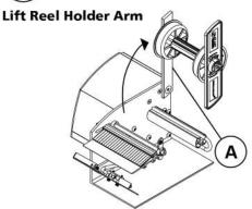
A: Lift reel holder arm slightly past 90° angle and lock into position using provided hex wrench
