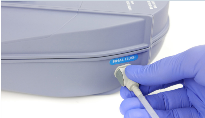
7 / Connect the Flush Tube at the back of the Station.
