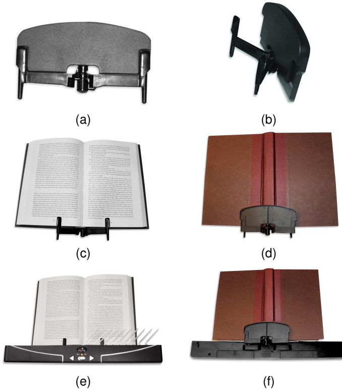
Figure 7: (a) Book clamp; (b) Pull spring-loaded arms outward to slide book between flexed arms and supporting plate. (c) Front and (d) rear view of book clamp with mounted book; (e) Front and (f) rear view of book/clamp assembly mounted on PageFlip Lite. Notice that clamp snaps into rear slots of PageFlip Lite.
