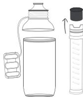
Prior to the first use of LifeStraw Play, remove the filter and the carbon capsule. Rinse all parts with clean water. Reassemble and LifeStraw Play is ready to use.
