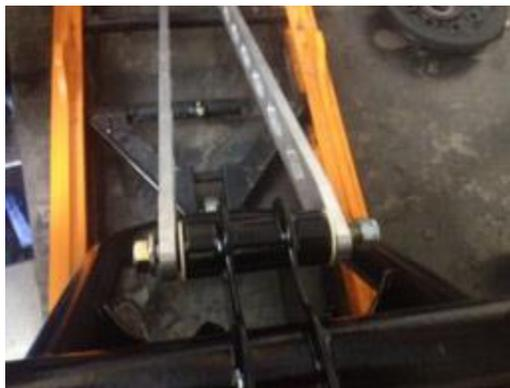
12. With the throttle rods mounted, install rear shock. Use 8 mm bolt and flange nut supplied. For ease of installation, install lower shock mount in rocker arm first. Do not tighten at this time.
