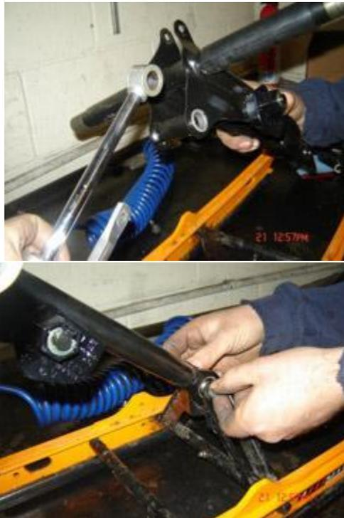
8. Remove stock rocker arm mounted to front Arm. Install new rocker arm with newly supplied bushings, using existing bolt and new 10mm nut provided with your E- Motion kit.
