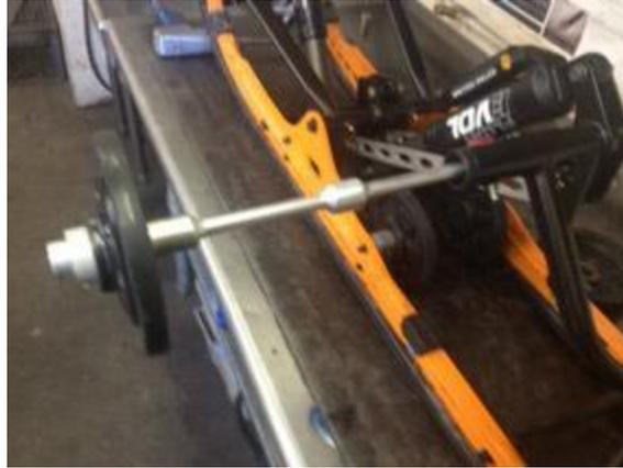
16. Loosen one or both (depending on year model), limiter straps by removing the bolts and nuts from the lower part of limiter strap. Remove upper shock bolt and lower shock shaft. Set bolt aside to be re-used during re-assembly.
