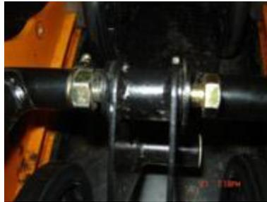
9. Install new E-motion rear arm attaching rear pivot first .Use existing bolt and new 8mm flanged nut. Torque rocker arm bolt to 35 ft. lbs.
