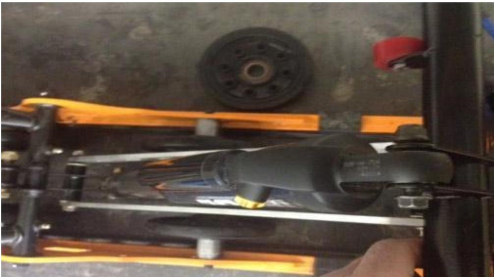
14. Torque shock and throttle rod bolts to 18 ft. lbs. Install new rear arm axle into E-Motion arm and install stock idler wheels and retaining rings. Use 242 Loctite on the 3mm Allen to prevent the screw from backing out.
