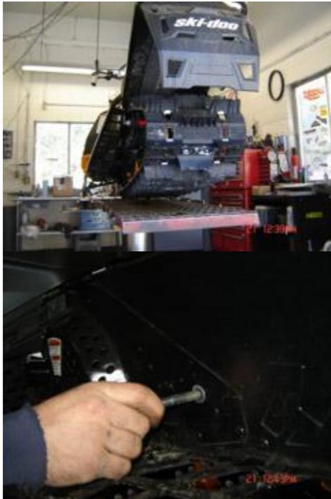
4. With the suspension free from the tunnel, remove the bushings and axles from the front arm. The front arm axle and bushings will be re-used during re-assembly.
