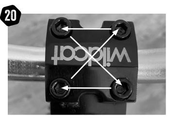
NOTE: Stem bolts need to be tight! Work around the bolts a few times to ensure it is securely tightened down. Each time you tighten one bolt it will allow you to get another partial turn on the other bolts. A lot of force is put through the stem when riding due to the amount of leverage on the bars, you don't want them to move!
