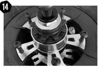
Replace the 5 x 3mm hex bolts and tighten down. Replace the axle washer and nut.
