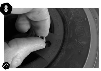
Insert rim hardware and tighten. Caution, tighten securely but do not over-tighten, the nylock will prevent them coming undone.
