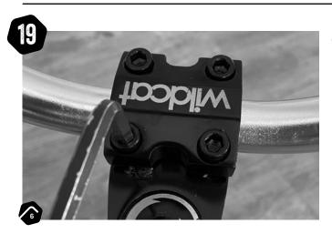
Once you're happy the bars are in the correct position and the plate is level, work diagonally opposite and tighten down each bolt.
