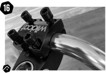
Insert the 4 x bolts, ensuring the bars stay centred in the stem.
