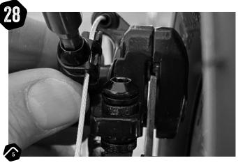
On the brake, pull the cable so the cable tube seats in both the lever on the handle and on the brake unit.
