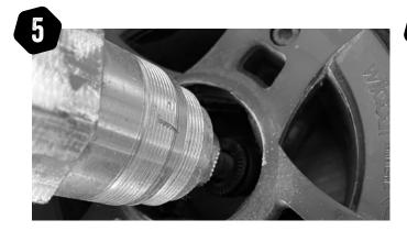
Flip the wheel over, and push down on the tyre / rim against the floor, the hub will simply slide out of the rim assembly.
