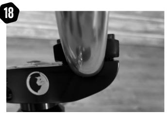
Check from the side to ensure the stem plate is parallel with the stem, the gap both sides should be equal. If not, back off the low side and slightly tighten the other.
