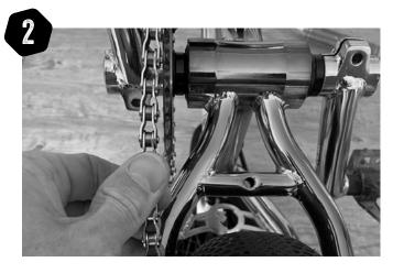
Slide the wheel forwards to release the chain, then slide the wheel out of the back of the frame drop-outs.
