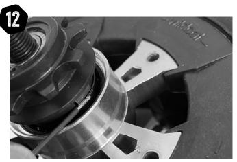
If the driver did pop out, place it back on the axle and holding the 3 x palls in gently rotate and push it back in.
