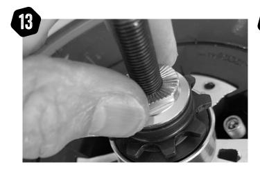
Replace the spacer and wind down to hold the assembly in place. Once together visually check the large spacer between the hub halves is correctly seated in both sides. It will have a little slop until you tighten down the 5 x 3mm hub bolts.
