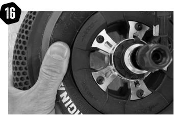
To adjust, squeeze the tyre and position on the rim. When you're happy add a little air to secure it then repeat on the other side.
