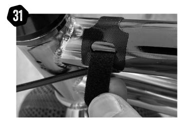
Secure the cable to the top tube at both ends, using the 2 x velcro ties.
