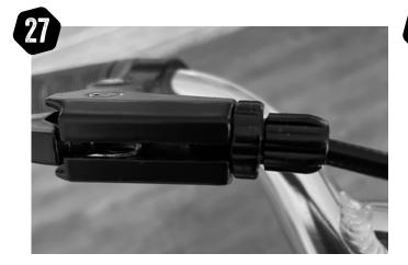
Tighten the cable adjuster barrels against the lever, ensuring to misalign the slots to prevent the cable escaping.
