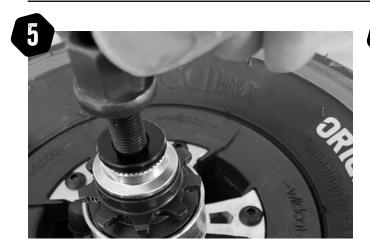
NOTE: ENSURE THE TYRE IS DEFLATED BEFORE **CONTINUING.** Remove the axle nut on the driver side only.
