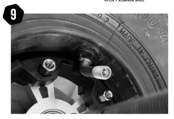
**REASSEMBLY:** Ensure the valve is correctly positioned and facing the driver side.
