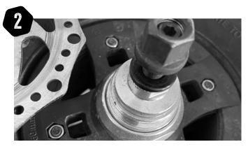
Once released / loosened the disc will simply wind off by hand.
