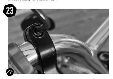
On the brake lever, loosen the hex clamp bolt with a 4mm allen key, position on the handle bars to suit and tighten.
