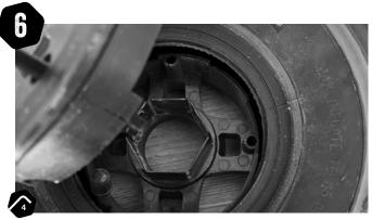
**NOTE: ENSURE THE TYRE IS DEFLATED BEFORE CONTINUING.** Undo the 4 x rim bolts using a 4mm allen key, then the rim will simply pull apart off the tyre.
