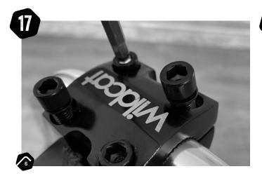
Lightly tighten down two diagonally opposite until it begins to pinch on the bars. Then rotate the bars up and tighten slightly more to hold them in place.
