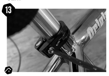
Position the seat at the desired height, and tighten the clamp using a 4mm allen key. Ensure the seat is aligned with the frame.
