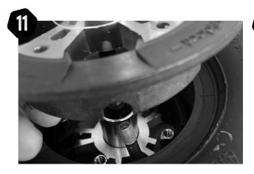
Replace the driver side onto the axle, again check to see the valve slot on this side is aligned correctly.
