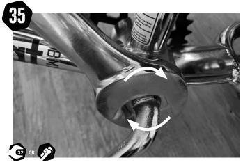
If adjustment is required back the 32mm nut off with a spanner or wrench. This is reverse thread, so clockwise to loosen.
