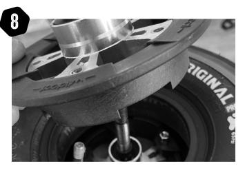
Due to the internal locking system you may need to slide the aluminium hub out of the rim, then work around the rim pulling up firmly with your hand to separate it. Once released both sides can be removed from the tyre, then you have access to change or fix the tyre.
