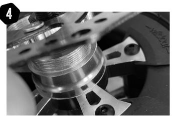
Once released / loosened the disc will simply wind off by hand.
