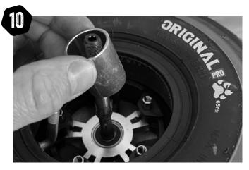
Take care to replace the large spacer and check it's seated correctly before reassembly.
