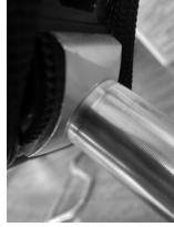
If you have a Pivotal seat, the seat angle can be adjusted with a 6mm allen key, through the slit on the top of the seat. Simply loosen, rotate to the desired position and tighten.
