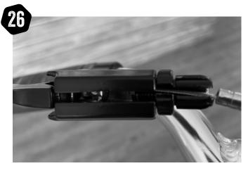
Place the cable into the slot as shown.
