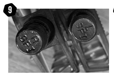
Pedals are marked 'L' & 'R' on the end of each spindle. **Original2** has a 1 piece crank and 1/2" thread pedals, **Pro-Series** has a 3 piece crank with 9/16" pedals.
