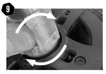
Insert the hub assembly, you will need to rotate back and forth as you push inwards to clear the inner flanges.
