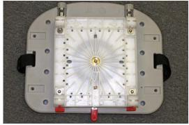
**13)** Rotate the swivel plate 45 degrees back to the proper locked position. The replacement is now complete.
