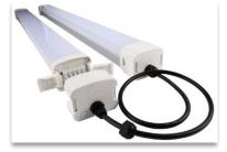
4. Make connection between the wires and quicker connector, black wire goes to L, green wire goest to G, white goes to N, Purple wire goes to dim+, and Gray wire goes to dimm-. Relock the junction box screw the end cap of waterproof connector
