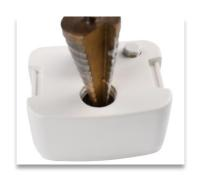
2. Install the sensor on the endcap by the lock nut
