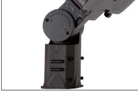
Slipfitter Mount An optional cast aluminum mast arm adapter secures fixture head to nominal 2-3/8" O.D. horizontal steel tenon arm.
