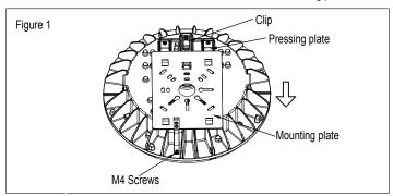
3.Connect the clip on the fixture to the spindle of the mounting plate to make sure the fixture will not slip and fall.connect the line voltage to the wires coming out from the fixture following the wiring diagram. Push the pressing plate into the suspension loop on the mounting plate. 2.Fix the mounting plate to the ceiling with the screws.
