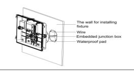
6.Connect the input wire and the dimming wire of the light, then put the connect ed wires into the embedded terminal box.
