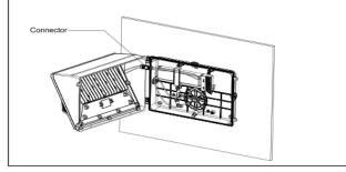
2.Unscrew the cover of the entry hole on the lamp base and remove the cover .
