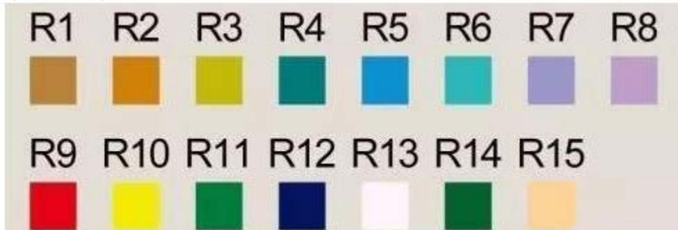
To estimate if the CRI of the light source is good or not, we see the value of it at the 15 points. When comparing a light source with a specified reference source, the index value of 100 is the best. Generally, the color rendering properties of light sources are roughly divided into four categories by CRI: Below 50 is "poor", 50 to 70 is "average", 70-80 is "good", and above 80 is "excellent".
