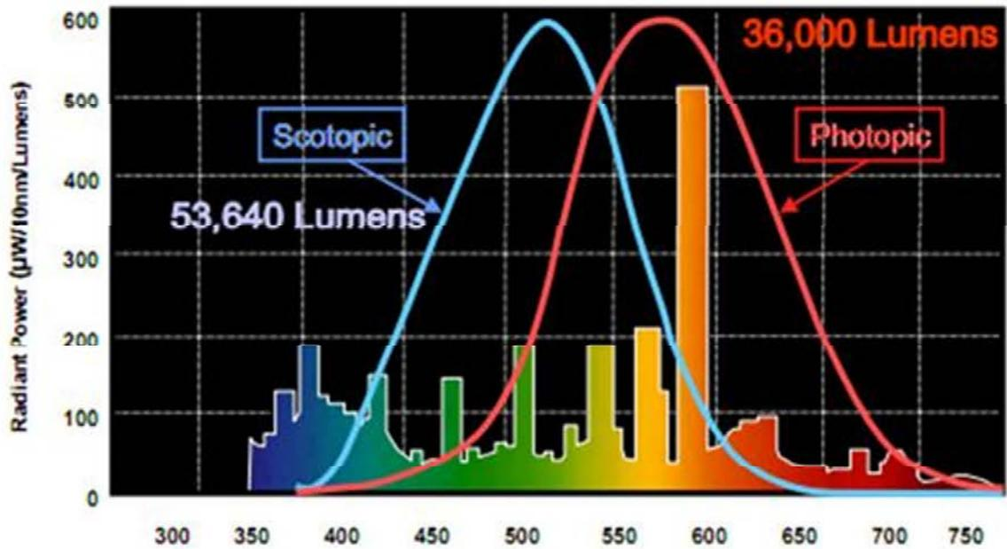
Once the S/P ratio is known, Pupil Lumens which are a more accurate estimate of the stimulation of the eyes by a particular light source can be estimated based on formulae developed by scientists at the Lawrence Berkley Laboratory (LBL).
