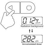
The transition between the radiation background measurement modes and the accumulated dose is carried out by briefly pressing the mode button
