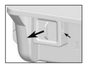
Press the side lock and remove the CAN dongle.
