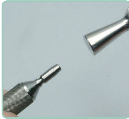
3.4 Placement of the abutment onto the specific handle for abutments, engaging the internal hexagon and applying an impulsive force. The handle facilitates the reduction of the abutment and prevents any damages to the abutment. It also avoids problems due to overheating and unstable grips.
