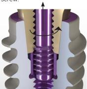
Gently lift up the driver while rotating it counter-clockwise to engage the screw in the internal threads of the abutment.
