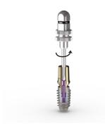
Using a .050 tapered hex driver, unscrew the fixation screw.
