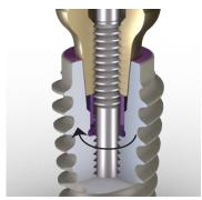
Continue to turn the abutment removal tool until the abutment releases from the tapered connection of the implant.
