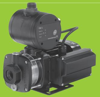
The BasicLine by Grundfos CMBasic is a compact booster pump designed for domestic and light industrial use. The booster unit consists of a Grundfos CM cast iron pump with stainless steel hydraulic components and PM1 Pressure Manager. The Pressure Manager allows the pump to start and stop automatically according to demand and protects the pump from dry running.
