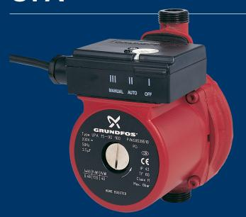
The UPA Homebooster is a circulator pump designed for pressure boosting hot water systems. The pump provides additional pressure to showers, taps and similar outlet points. The UPA Homebooster is for use in open systems. The pump incorporates a flow switch which starts or stops the pump when a tap is turned on or off.
