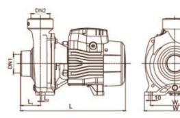
DN1 DN2 L (mm) W (mm) H (mm) L1 (mm) L2 (mm) W1 (mm) 2' 2" 371 263 3.5 206 59 166
