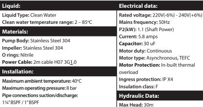
Max Flow: 204 l/min
