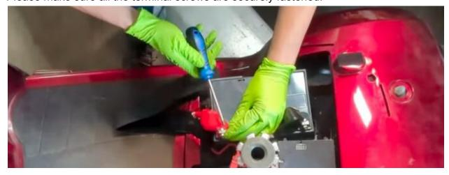
8. Secure the batteries with the original straps or other methods to ensure the battery does not move around.
