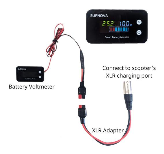
Your mobility kit's battery meter should come pre-calibrated to match your batteries and is connected via the XLR adapter to your mobility scooter's XLR charging port.
