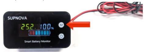
2. You should see the sub-menu below. Short Press the "M" button until you see #3 as shown below. Then press the "Power" button below once.
