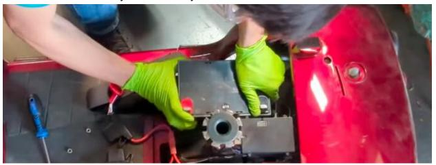
6. Place the new lithium batteries. Most mobility scooter's cabling will already be set up for series connection and you just need to connect the original cabling: red cable to the red terminal (+) and black cable to black terminal (-) on each battery.
