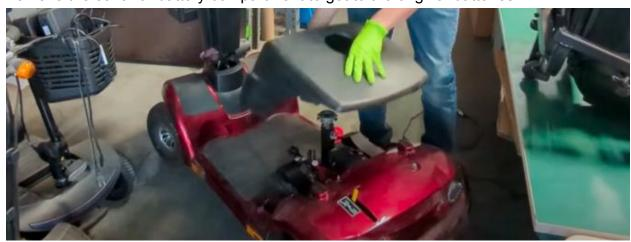
3. Take a few pictures of the original cabling. (in case needed for reference) Please note, if your batteries are in "Series" or "Parallel" connection. Most mobility scooters will use two 12V batteries and are set up for "Series" connection.
