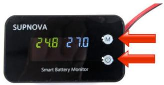
5. Once you have the voltages you wanted, long press the "Power" button to save the settings. The numbers should stop blinking and be solid.
