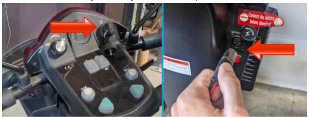
2. Remove the cover or battery compartment to get to the original batteries.
