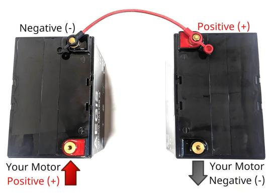
The diagram above demonstrates "Series" connection for batteries. In series, the voltage is doubled to meet your application motor needs. For example, two 12V batteries connected in series will output 24V to your motor.
