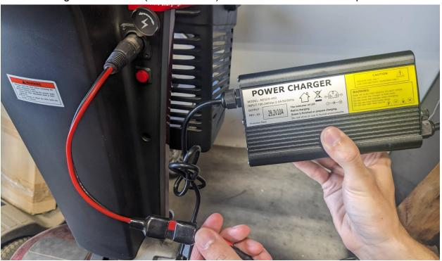
2. If the XLR cable is not connected already, you can connect the XLR cable to the charger by connecting the PP45 connections together via the adapter cable.
