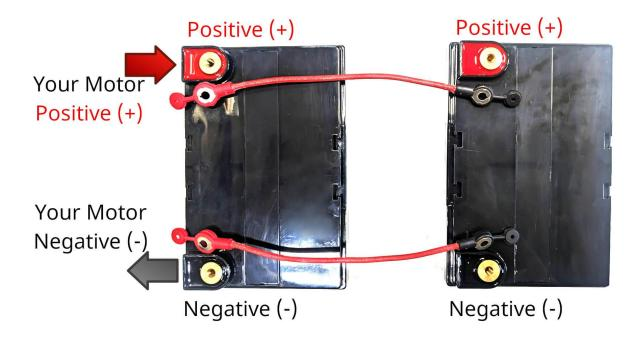
The diagram above demonstrates "Parallel" connection for batteries. In parallel, the amp hour is doubled to extend your battery capacity. For example, two 12V 25Ah batteries connected in parallel will output 12V 50Ah to your motor.
