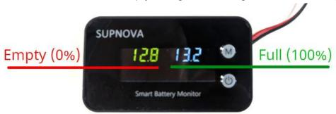
4. To cycle through the voltage numbers, short press the "M" button. Once you reach the number you wanted, short press the "Power" button to move to the next number column.
