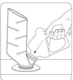
5. Insert nozzle. Before fueling, be sure the nozzle is inserted as far into the receiver as possible, making tight contact with the adapter.
