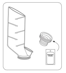
1. Choose the Deck Fill Adapter that fits your boat. Apply a thin coating of sealant to the rubber adapter threads. Do not over apply. Wipe off any excess with the enclosed alcohol towelette.
