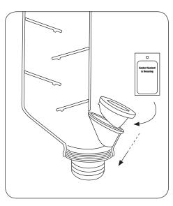
3. Apply a thin coating of sealant to the outside of the Nozzle Adapter and insert. Do not over apply. Wipe off any excess with the enclosed alcohol towelette. The larger opening is for diesel fuel nozzles, the smaller is for gas. The smaller adapter will also expand to fit tightly around different sized diesel nozzles.
