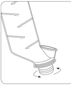
2. Force Deck Fill Adapter into the bottom of the baffle. Give it a few turns to seat it. Let sit for 12 to 15 hours before use.
