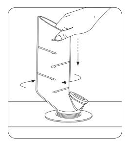
4. Push Clean Way down into boat deck fill and twist to seal tightly.
