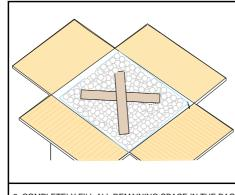
3 COMPLETELY FILL ALL REMAINING SPACE IN THE BAG WITH VERMICULITE, SEAL BAG WITH 75MM ADHESIVE TAPE.
