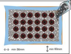
Place plastic liner bag inside box and add a minimum base layer of 55mm vermiculite before placing your inner product(s) into the box ensuring minimum spacing as shown
