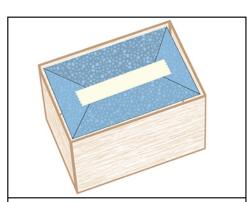
Completely fill all remaining space with vermiculite ensuring a minimum layer of 55mm vermiculite at the top of the box. Seal bag with 75mm adhesive tape.
