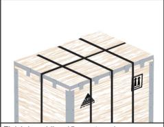
Finish by adding 15mm strapping to the box as shown.
