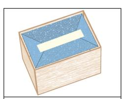
Completely fill all remaining space with vermiculite ensuring a minimum layer of 42mm vermiculite at the top of the box. Seal bag with 75mm adhesive tape.
