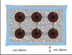
Place plastic liner bag inside box and add a minimum base layer of 38mm vermiculite before placing your inner product(s) into the box ensuring minimum spacing as shown
