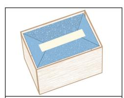
Completely fill all remaining space with vermiculite ensuring a minimum layer of 38mm vermiculite at the top of the box. Seal bag with 75mm adhesive tape.
