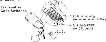
**▲** Warning! CFL bulbs are not applicable to the remote with dimming function.
