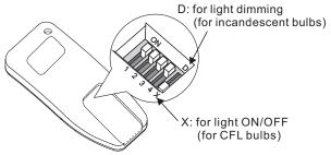
**Note:** You may switch Light switch code at D position (DIMMING) when you change to incandescent bulbs for Down light. To use dimming, press and hold light button(s).
