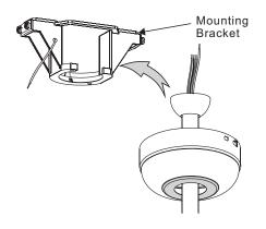
Rotate fan so that the groove on the ball engages the ridge in the mounting bracket.
