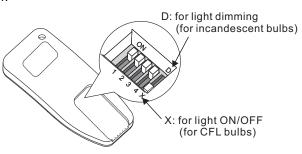
**Note:** You may switch Light switch code at D position (DIMMING) when you change to incandescent bulbs for Down light. To use dimming, press and hold light button(s).
