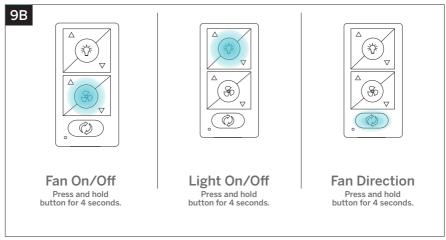
Fan On/Off: Press and hold  $\Re$  button for 4 seconds. The LED on the remote will flash green and all connected fans will beep to indicate the message has been received. All fans will turn off. This will bring all fans controlled by the remote into sync.
