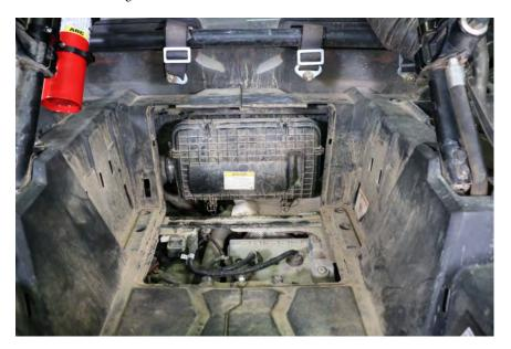
2. Release the four clips holding the air box lid on the air box.
