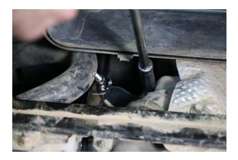
15. Tighten the boot connecting the intake pipe to the airbox.
