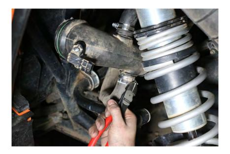
8. With the intake removed from the machine, remove the MAP sensor from the intake tube.
