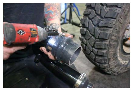
12. With the factory clamps placed loosely on the intake pipe boots, install the intake pipe onto the air box and turbo. It helps to get the small boot started and rock the pipe up towards the air box.
