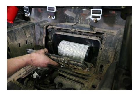
3. If you are using the kit with replacement air filter, remove the air filter now.
