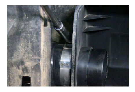
16. If you have the kit with the filter install the filter now. If not re install the factory filter now. Reinstall the air box lid and engine cover.
