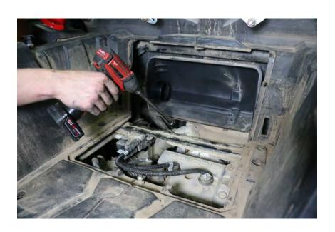
5. Loosen the clamp holding the boot to the air box inlet.
