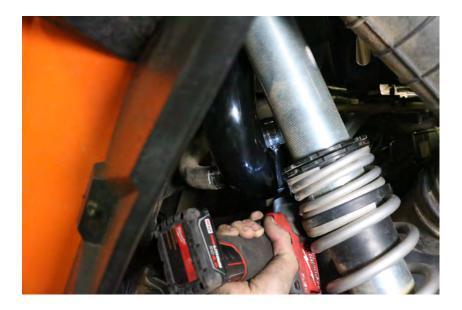
14. Tighten the clamp on the inlet of the turbo.
