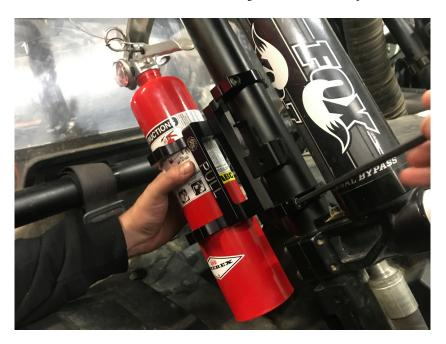
6. Firmly pull the "PULL" handle to remove the fire extinguisher from the base. Tighten the clamps to the base now.
