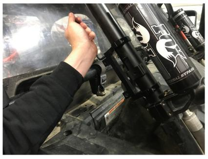
7. Reinstall the "PULL" handle with the fir extinguisher in place and the install is done. With this two pin design, you will have to make sure the "PULL" handle is aligned perfectly to put it back in. The Tight tolerances ensure there is not rattling of the fire extinguisher.
