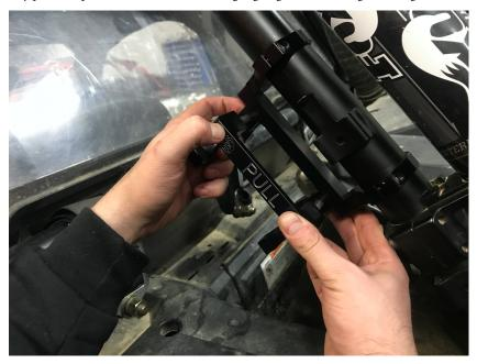
4. Now place the fire extinguisher into the base of the 3" clamps and install the top part of the clamp. You can tighten these four screws now.
