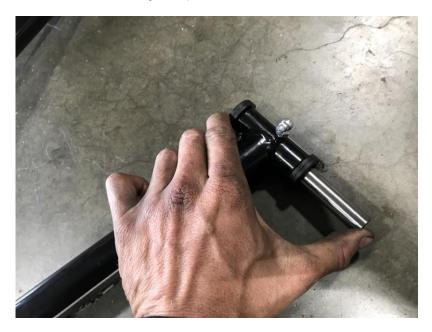
11. Place the arms in to the frame and install the factory hardware.
