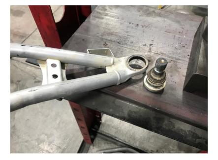
7. Install the ball joint into the new Deviant control arm.
