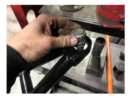
8. Using a press or vise press the ball joint into the new arm. Use large sockets or tube to press it in.
