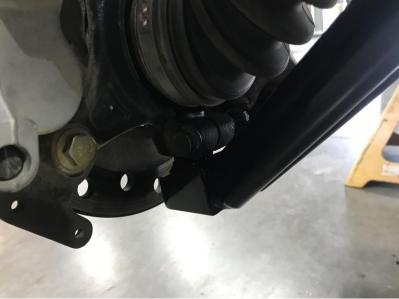
14. Grease both front and rear joints. Repeat process for the other side.
