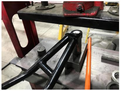
9. Install the snap ring onto the ball joint. If the snap ring wont seat tap the back of the ball joint with a dead blow to seat it completely.
