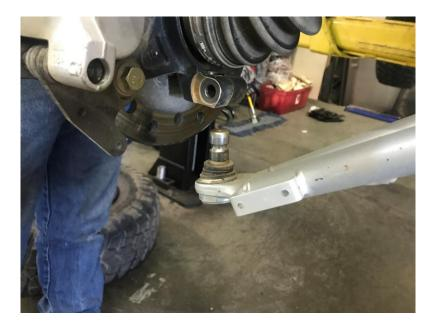
3. With 15mm tools remove the front and rear bolts from the control arms.
