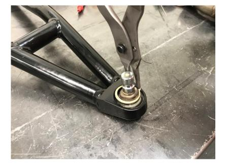
10. Install the new bushings and pin into the control arms.
