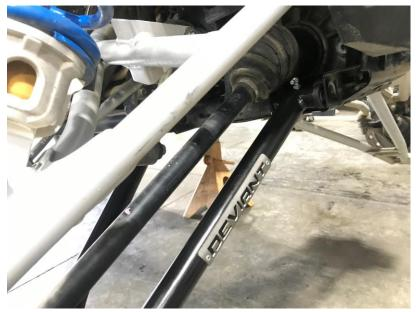
12. Tighten the front and rear frame bolts on the control arms. Torque to 42 foot pounds.
