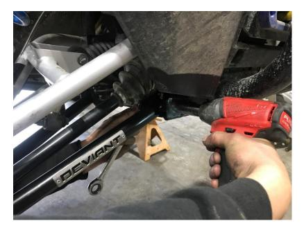
13. Place the ball joint into the spindle and install the bolt. Torque to 42 foot pounds.
