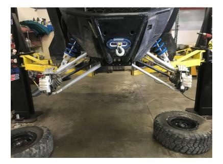
2. Using 15mm tools remove the lower ball joint bolt and remove the ball joint from the spindle.
