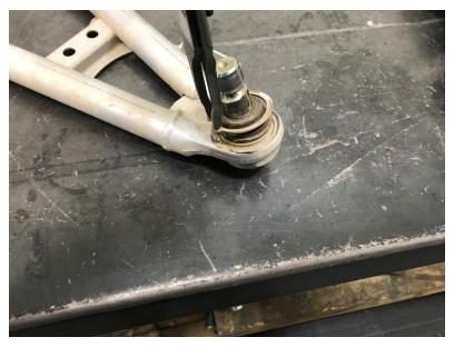
6. Using a press or vice use large sockets or tubing and press the ball joint out of the factory control arm.
