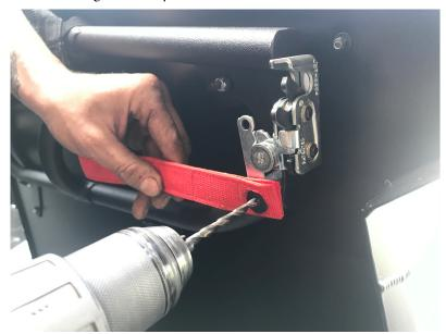
2. With the tether removed use the supplied hardware and install the new door handle as shown.
