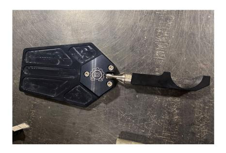
5. Place the clamp cap on the roll bar with threaded holes facing away from the windshield.
