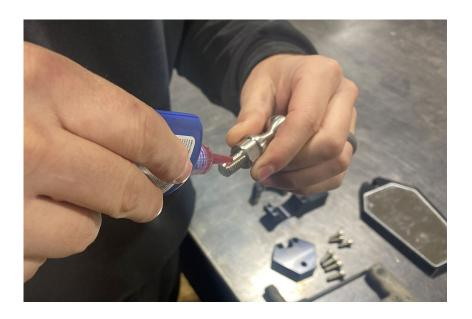
2. Thread the ball stud into the clamp and leave loose. This will be tightened once its on the machine.
