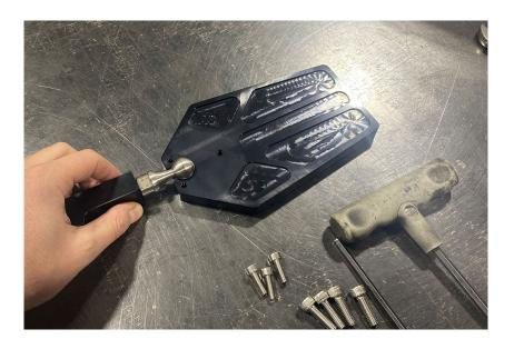
4. Place the mirrors back cap over the ball stud. Loosely install the three  $4\mathrm{MM}$  screws into the mirror.
