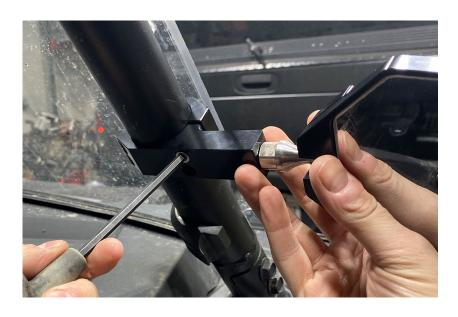
7. Now that the roll bar clamp is tight you can now tighten the ball stud with a 14MM wrench.
