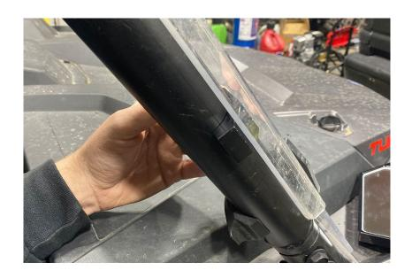
6. Install the four 5MM screws into the roll bar clamp, and tighten after it's placed in your desired location.
