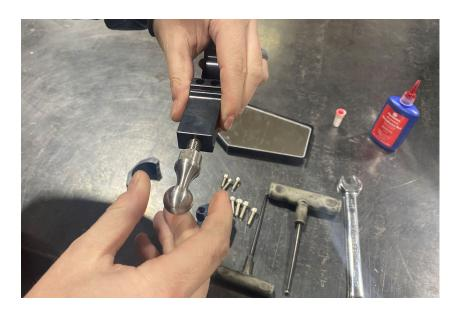
3. With the mirror side down. Place the ball stud into the pocket as shown.
