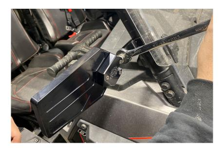
8. Loosely tighten the screw shown first on the back cap. Then loosely tighten the two screws closest to the roll bar clamp evenly. The screw thats furthest away from the roll bar should press the back cap against the mirror. Once the mirror is adjusted to the desired position tighten the two screws closest to the roll bar clamp.
