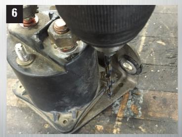
Remove the grid heater solenoid from the battery tray and drill two 3/16" holes in shown locations.
