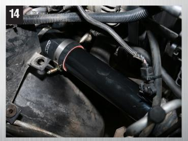
With compressor housing and charge air elbow loose maneuver the intercooler pipe onto the elbow and into the intercooler.
