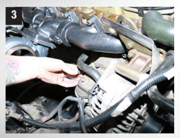
On the side of the oil filter housing remove the factory turbo oil feed line and fitting and install provided plug.
