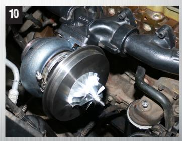
Now install the center cartridge of the turbo with the compressor housing removed. Be sure the oil feed and drain locations are perfectly vertical before tightening.
