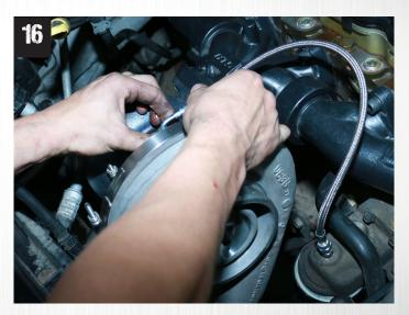
Install provided 4 AN oil feed line on the oil filter housing to the turbo as shown.
