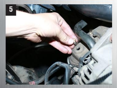
On the top of the oil filter housing remove the 1/8" NPT plug and install the new oil feed fitting.
