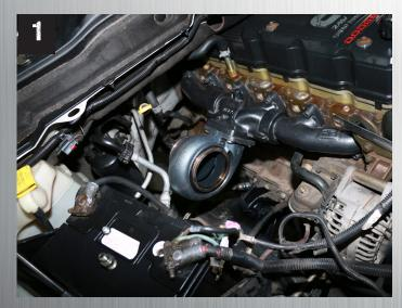
Start by installing the T4 Exhaust manifold with provided gaskets and hardware.
