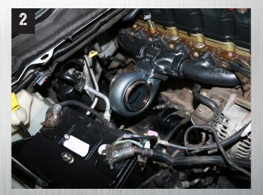
We like to install the turbo in pieces. Pictured is the turbine housing removed then installed onto the manifold with provided T4 gasket and hardware.
