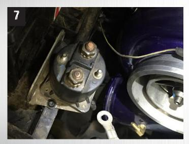
Relocate the grid heater solenoid to the top edge of the battery tray and drill two 3/32" holes into the battery tray. Use the two factory bolts to fasten the solenoid to the battery tray.
