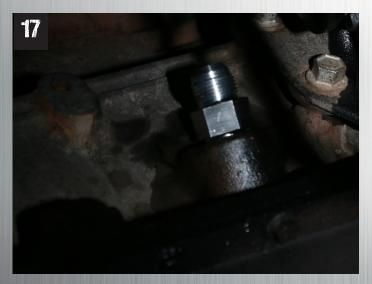
Install the 10AN oil drain fitting into the existing oil return location in the block.
