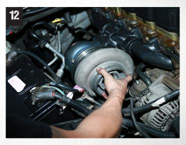
Install the compressor housing onto the turbo.
