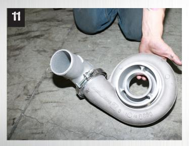
Install the cast charge air elbow onto the compressor housing with provided clamp and o ring and leave loose.
