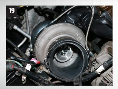
Install the molded intake hose, steel intake pipe and air filter with provide clamps.
