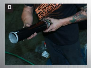
Slide the provided intercooler boot and clamps onto the intercooler pipe.
