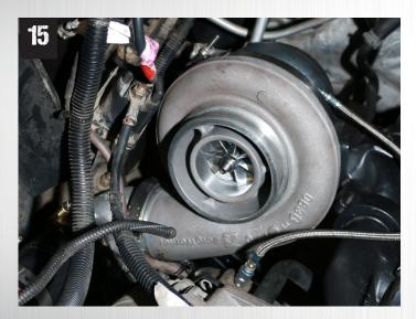
Once the intercooler pipe is installed tighten the compressor housing, charge air elbow, and intercooler boot clamps.
