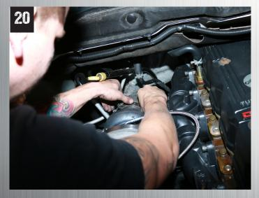
Install the down pipe onto the turbo with provided clamp then hook up to existing exhaust with the stainless steel band clamp.
