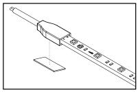
Use the Double-sided 3M Tape to secure the connector end.
