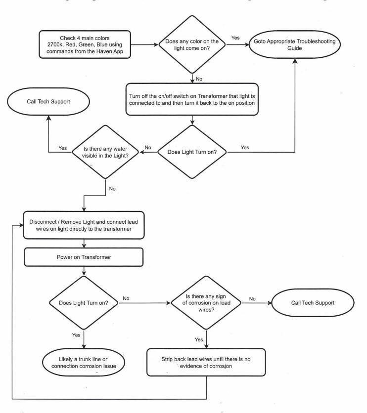
A good indication of a corroded wire is when lights are all off the voltage at the light connection (with light connected) measures normal (i.e. 15 VAC) and when lights are commanded on the voltage drops very low (i.e. 3VAC)
