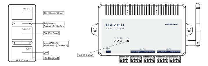
Tap the pairing button on the controller to pair a switch or change other settings. The controller will turn off both lights and the green status LED will turn off. Now that you are in pairing mode you can execute the following commands:
