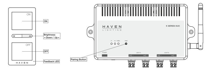
Tap the pairing button on the controller to pair a switch or change other settings. The controller will turn off both lights and the green status LED will turn off. Now that you are in pairing mode you can execute the following commands:
