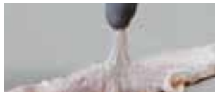
Filaments appear on the finger when adhesive layer is touched after ca 5 min. → optimal adhesive bond
