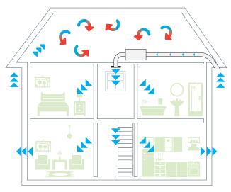
If the loft temperature is above 24°C air is drawn directly from outside, to provide background ventilation. In addition a boost switch is supplied to increase airflow when required.
