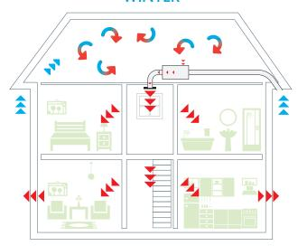
During the colder months tempered air is drawn from the loft space taking advantage of solar gain combined with the heat conducted through the ceiling of the home.
