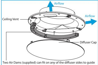
airflow away from a smoke detector and/or obstructions as required.
