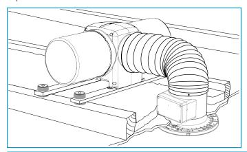
Place anti-vibration mounts above and below each batten fixing point and, using the 4 large screws and special washers, fix the unit to the joists.
